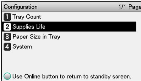
4 Select the consumable or maintenance unit (image drum, belt unit, fixer unit, or waste toner box) to be checked.
