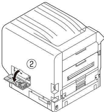
**3** Check that the internal LED lamp (①) is OFF.
