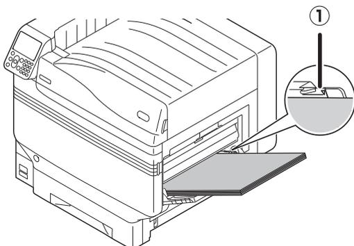
**7** Adjust the paper guide to fit the width of the paper that has been set.
