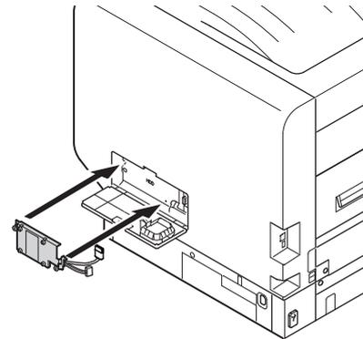
**5** Rotate the screws (x2) in the direction of the arrows to tighten securely.
