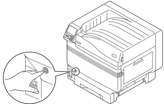
"Shutting down. Please wait. Power will turn OFF automatically" will be displayed in the control panel, and the power switch LED lamp will flash on an approx. 1-s cycle.
