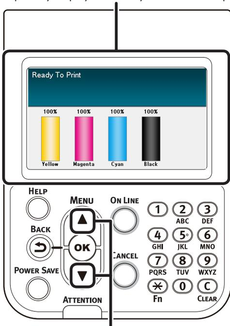
Press the scroll button ▲ or the ▼ to display the "Functions" menu screen as shown on the right.
