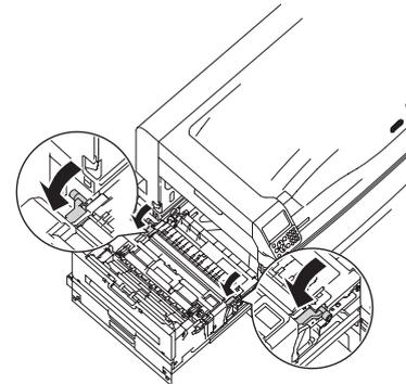
**6** Put the exit unit back into the printer.
