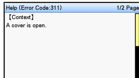
Press the ▲ scroll button displayed in the help screen to scroll to the previous page. Press the ▼ scroll button to scroll to the next page.
