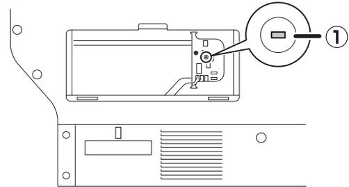
**4** Align the screws (x2) on the built-in HDD to the holes on the device.
