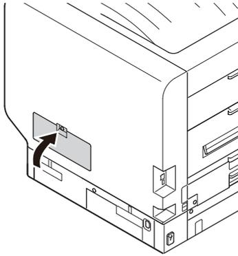
**8** Tighten the access cover screws.
