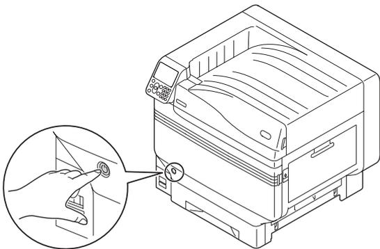
"Shutting down. Please wait. Power will turn OFF automatically" will be displayed in the control panel, and the power switch LED lamp will flash on an approx. 1-s cycle.
