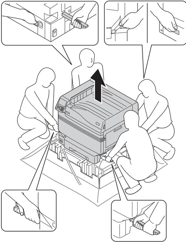
**5** Gently lower the device into its installation location.
