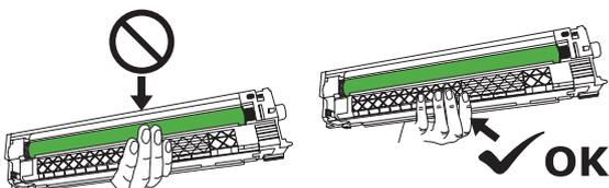
**3** Place the image drum that has been removed onto a flat surface covered with paper, and remove 4 stoppers (orange) in the direction of the arrows.
