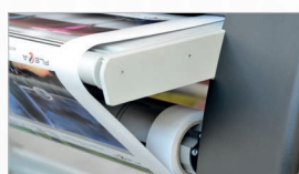
Removable steel worktop on ball bearing system for easy loading of materials
