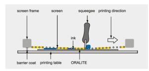
For printing, it is recommend maintaining a medium squeegee speed of approximately 0.75m/s [2.5 ft/s] and the squeegee should be applied at an angle of 30° to the print surface.
