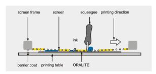
For printing, we recommend maintaining a medium squeegee speed of about 0.75m/s and the squeegee should be applied at angle of 30° to the print surface.
