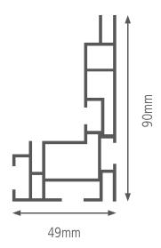
This aluminum profile is specifically designed for illuminating large format textile printing. With a smart design with multi-channel profile is this frame suitable for wall mounting as well as for standing and hanging solutions. Combined with our High PowerLED modules perfect wall light arises.
