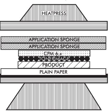
Note: Press smaller PLANX products for 1 minute, larger products for 1.5 to 2 minutes. Let the surface cool down for 20 to 40 seconds (depending on how long you have pressed before) before stripping off the paper!
