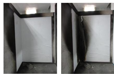
Before Test (EN 13823) After Test (EN 13823) SGS authenticate the photos on original report only Note: The above test was carried out by SGS-CSTC Standards Technical Services Co., Ltd. Shunde Branch. \*\*\*\*\*\*\*\*\* End of report\*\*\*\*\*\*
