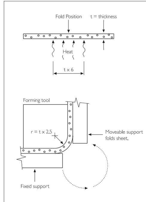
When using Electrical Heated Metal Tracks, the following guidelines should be adhered to:
