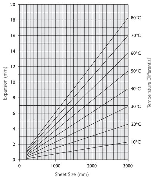
Foamalux can be used in conjunction with many common building and accessory materials; the thermal expansion properties of which must also be taken into consideration. The graph on the right illustrates the relative coefficients for various materials. Foamalux clearly expands much more than timber, concrete, brickwork and metals when their temperature is changed by the same amount.
