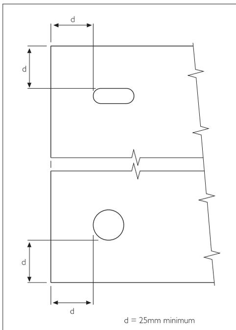
Fasteners should be spaced at the separations given for each thickness of panel.
