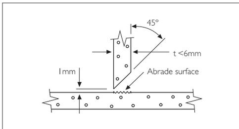
DOUBLE BEVEL BUTT WELD
