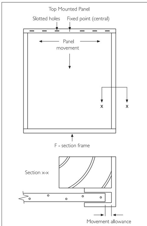
maintain a ventilating air gap of about 20mm behind the panel. Direct mounting of the panels to the walls could result in distortion due to heat build up.
