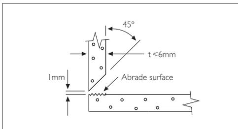
SINGLE BEVEL BUTT WELD
