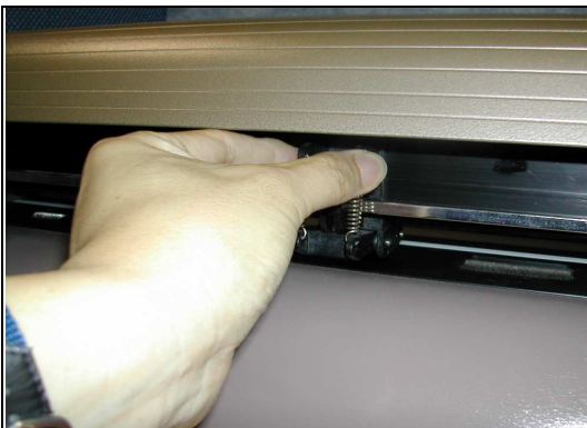
Figure 4-3 correct way to move pinch rollers
