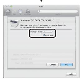
11 Check that [OKI DATA CORP C931] is displayed as added to the printer list, and close the "Print & Scan" screen.
