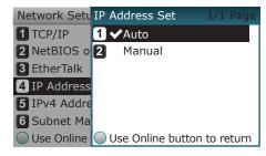
Press the scroll button ▼ several times to select [IPv4 Address], and then click the [OK] button.
