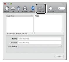
10 Select the printer, and check that [OKI C931(PS)] is displayed in [Print Using].
