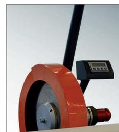
Digital control for precise cutting blade positioning
