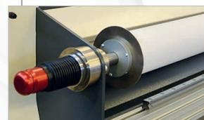
Shaftless unwind system for rapid master roll changeover
