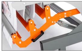
Pneumatic counterbalanced buffering system: it keeps the media always tensioned avoiding tears
