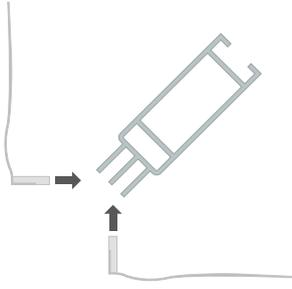
Place the textile print in the frame. Start with the corners and press the silicone strip in the channel.
