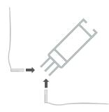
Place the textile print in the frame. Start with the corners and press the silicone strip in the channel.
