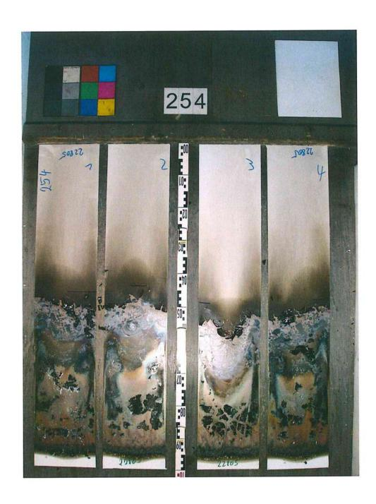
Picture 1: Appearance of specimen A3 after the test
